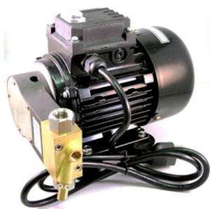
A direct drive mist pump assembly for commercial or residential installations. Low noise level makes it easy to work with Features auto water shut off. Internal adjustable pressure regulator (200-1000 PSI max.) Has 1– 12 mist nozzle capacity.
